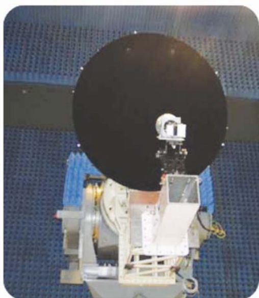
Figure 7. HGA in high power testing.
