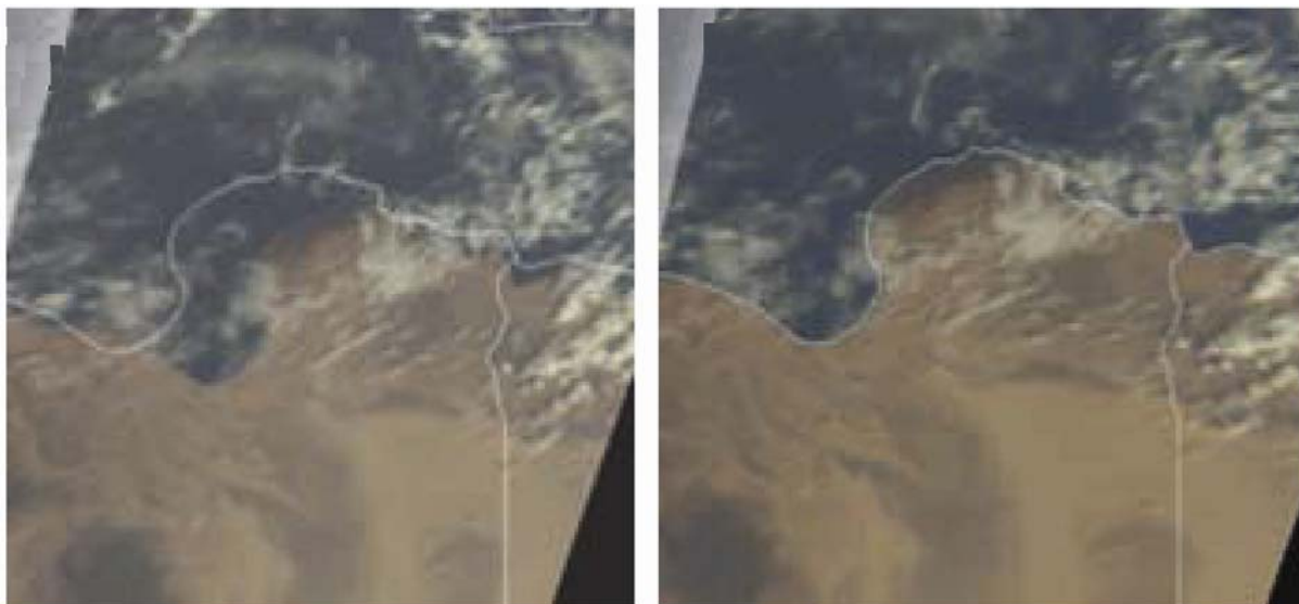
Figure 18. Images showing match between coastal and land boundary before (left) and after (right) improvement.
