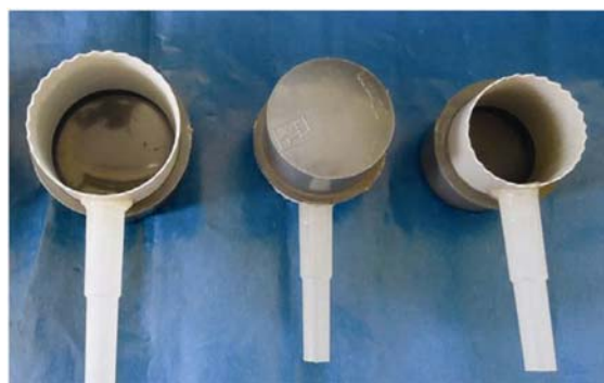
Figure 3. PVC connectors of different sizes attached with a hard tube.
