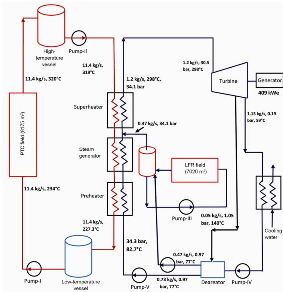
Figure 10. Heat and mass balance diagram of the plant for the time duration 14.00–15.00 on 4 June 2014.
