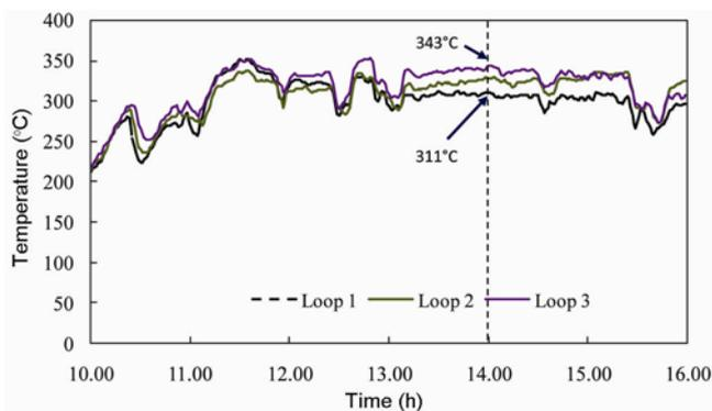
**Figure 12.** Typical loop imbalance problem in PTC field (4 June 2014).
