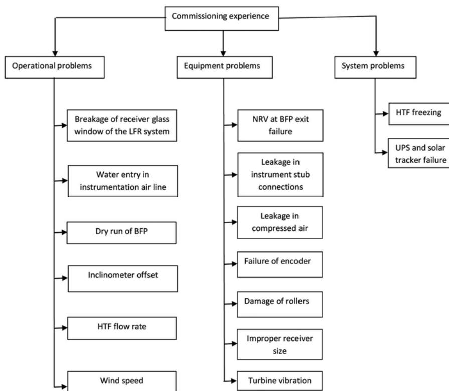
Figure 7. Experience in commissioning of solar thermal power plant.
