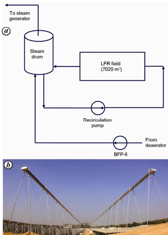
Figure 4. a, Schematic diagram of Linear Fresnel reflector (LFR) field. b, LFR field installed at site.
