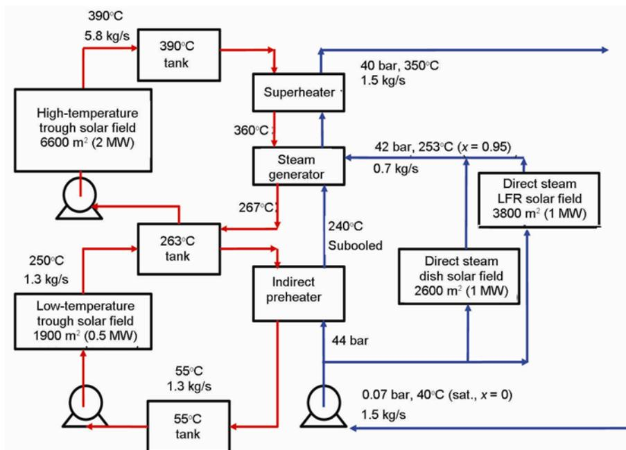
Figure 1. Schematic diagram of the proposed configuration.
