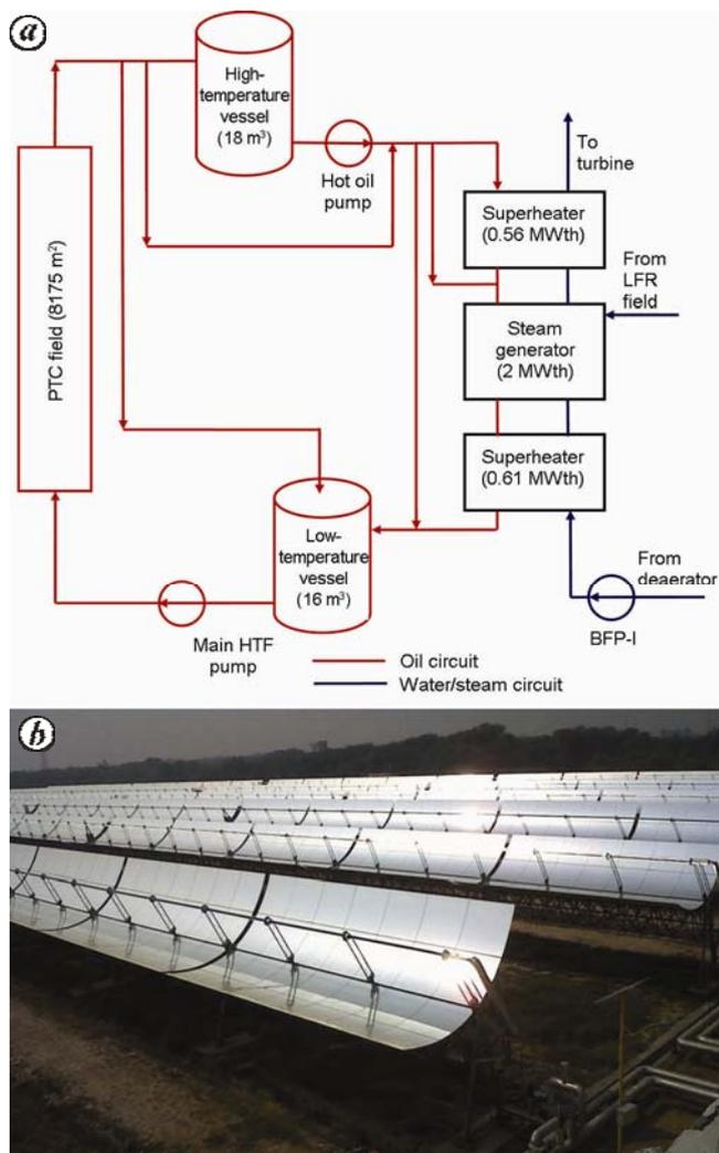
Figure 3. a, Schematic diagram of parabolic trough collector (PTC) field. b, PTC field installed at site.
