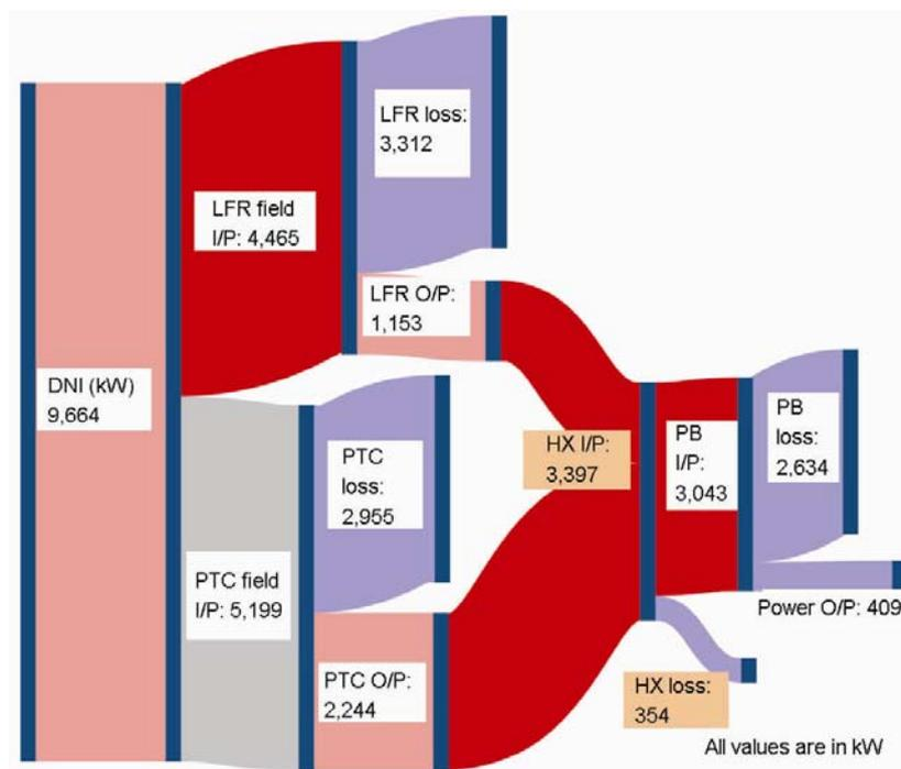
Figure 11. Sankey diagram for the time duration 14.00–15.00 on 4 June 2014.
