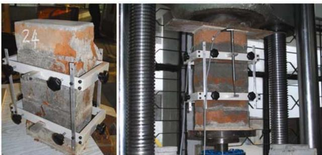
**Figure 3.** Set-up for carrying out test on compression behaviour of brick masonry specimen.
