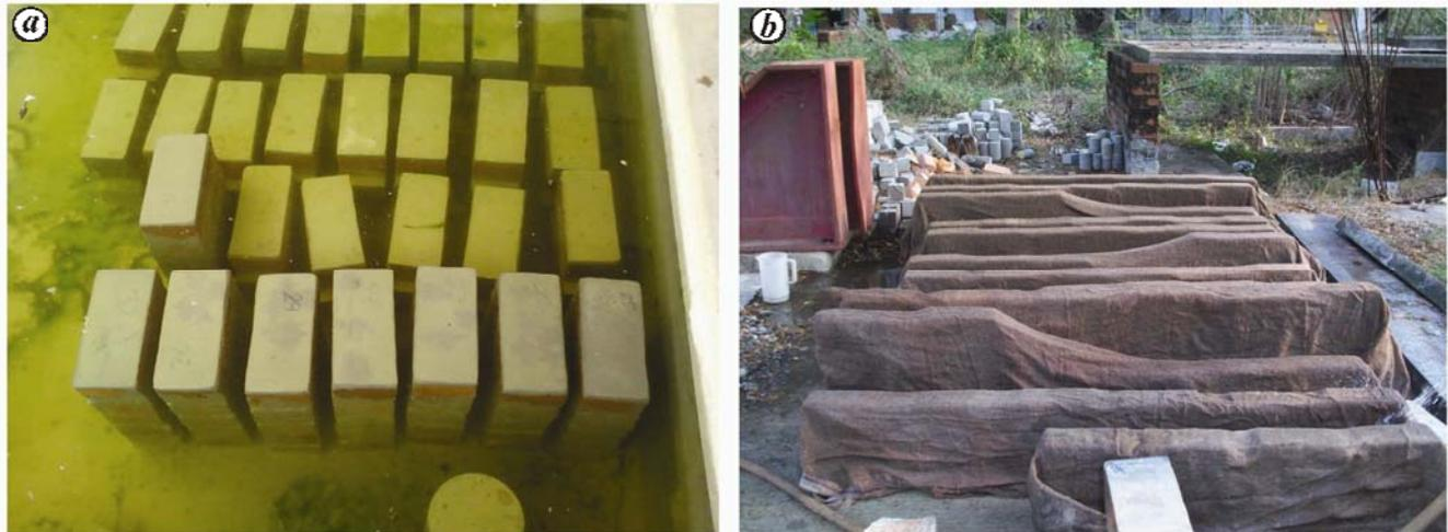
**Figure 2.** *a*, Curing of fabricated specimen under water up to 7 days. *b*, Curing of specimen under wet burlap during 8–28 days.
