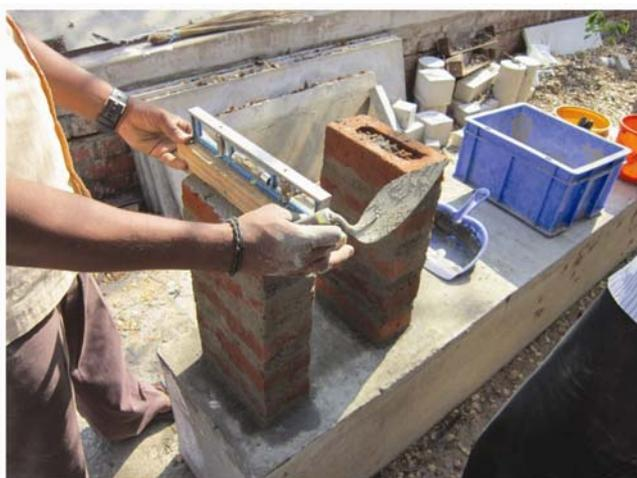
**Figure 1.** Fabrication of bricks masonry stack bonded prism.
