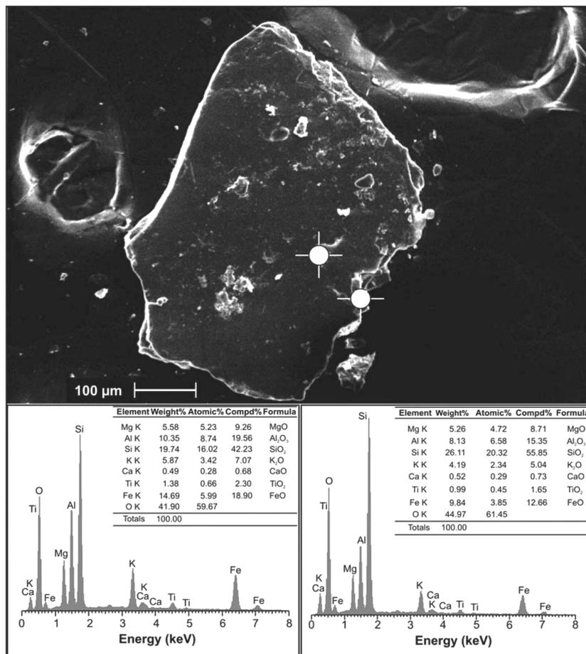
**Figure 2.** (Upper) Scanning electron photomicrograph of biotite grain of S1 sediment sample. The grain margin shows the effect of weathering as exfoliation and dissolution. (Lower) Results of Energy Dispersive X-ray (EDX) analysis of unweathered surface (a) and weathered surface (b) of the biotite grain. Peaks are levelled with the EDX line of the corresponding element and elemental data (in table) are presented in both weight and atomic per cent.
