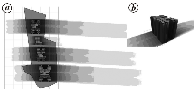
Figure 5. a, b, Ecotect: shadow analysis (G + 10) apartment in Coimbatore.
