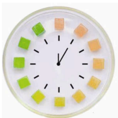
Figure 2. Photograph of the hydrogel cubes ( \sim 5 \times 5 \times 3 \text{ mm}^3 ) arranged in a manner resembling a clock in a petri dish, illustrating the red-to-green chronochromic performance. Reprinted with ACS permission from Zhang et al. 7 . Copyright (2014) from the American Chemical Society.
