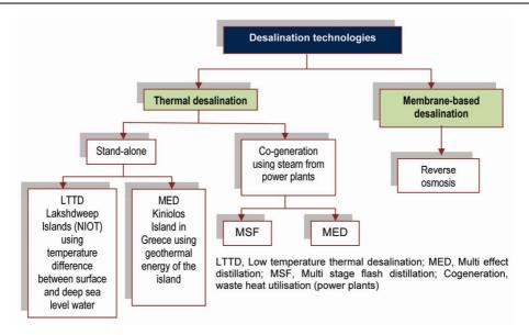
Figure 1. Desalination technologies. Source: Ref. 10.
