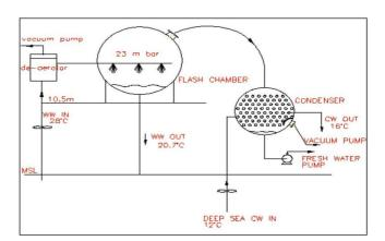
Figure 2. Schematic of LTTD process for Karavatti. WW, Warm water; CW, Cold water. Source: NIOT, Chennai.
