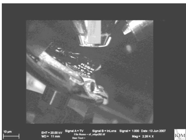
Figure 2. Pottery mounted in SEM chamber for characterization.
