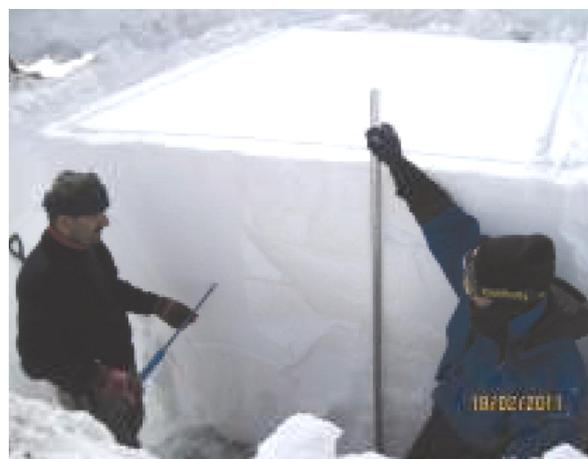
**Figure 2.** Snowpack dielectric profiling using snow fork.
