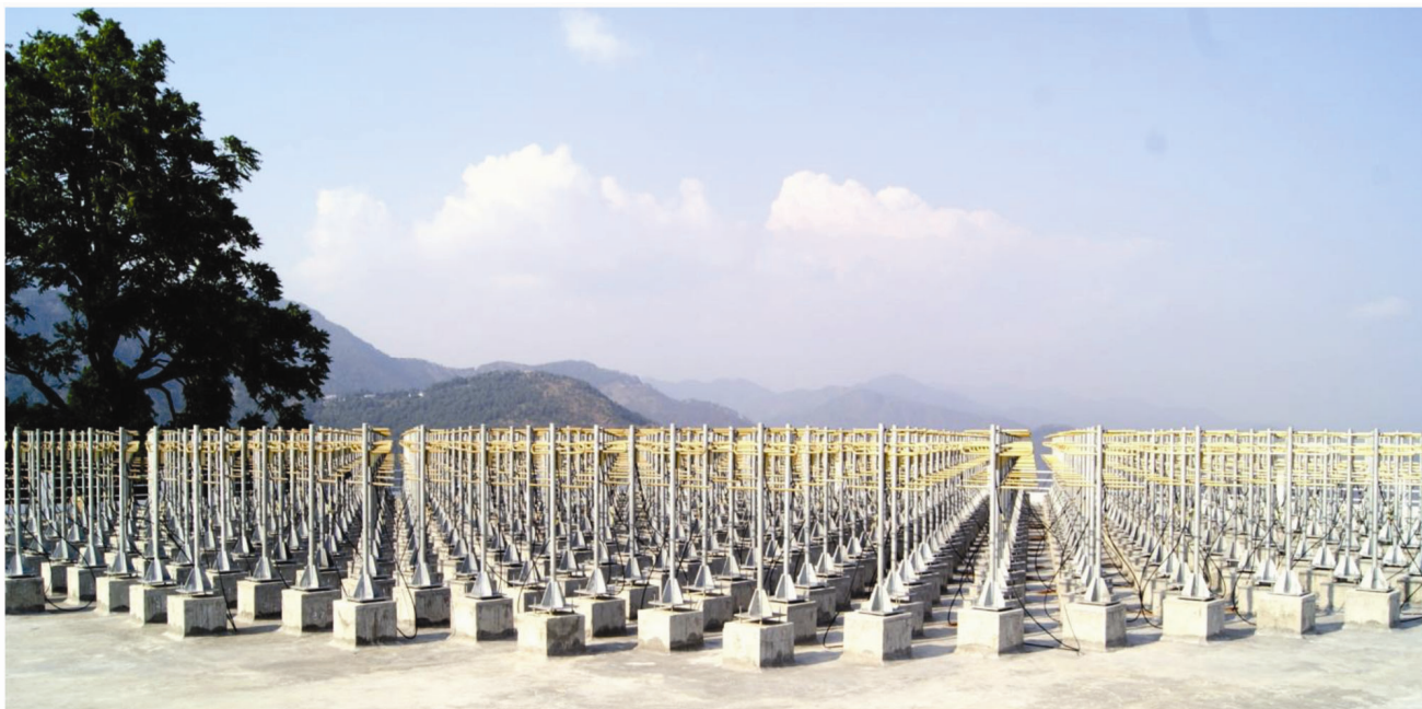
Figure 11. Antennae array of stratosphere–troposphere radar on the rooftop of the building at ARIES.
