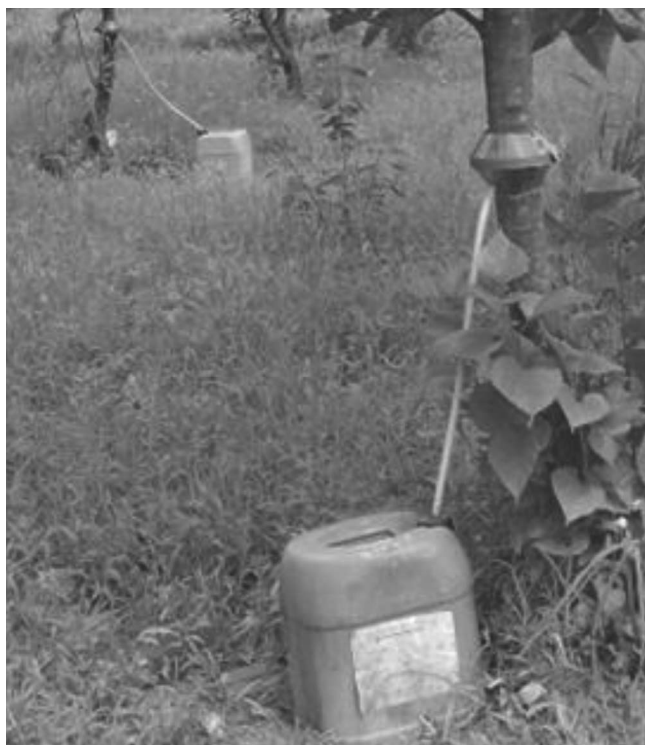
Figure 2. Instrumentation for measuring stemflow.
