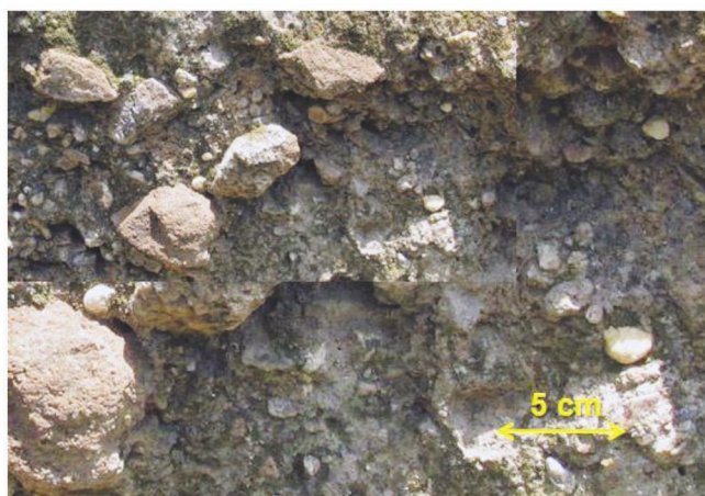
Figure 12. Soil profile section at a trench near Jain ‘basadi’ showing cluster of materials, including broken fragments of bricks and stones of different sizes and shapes as well as well-rounded, small-sized pebbles of quartz of varying sizes embedded in fine-grained mixture of silt and clay.
