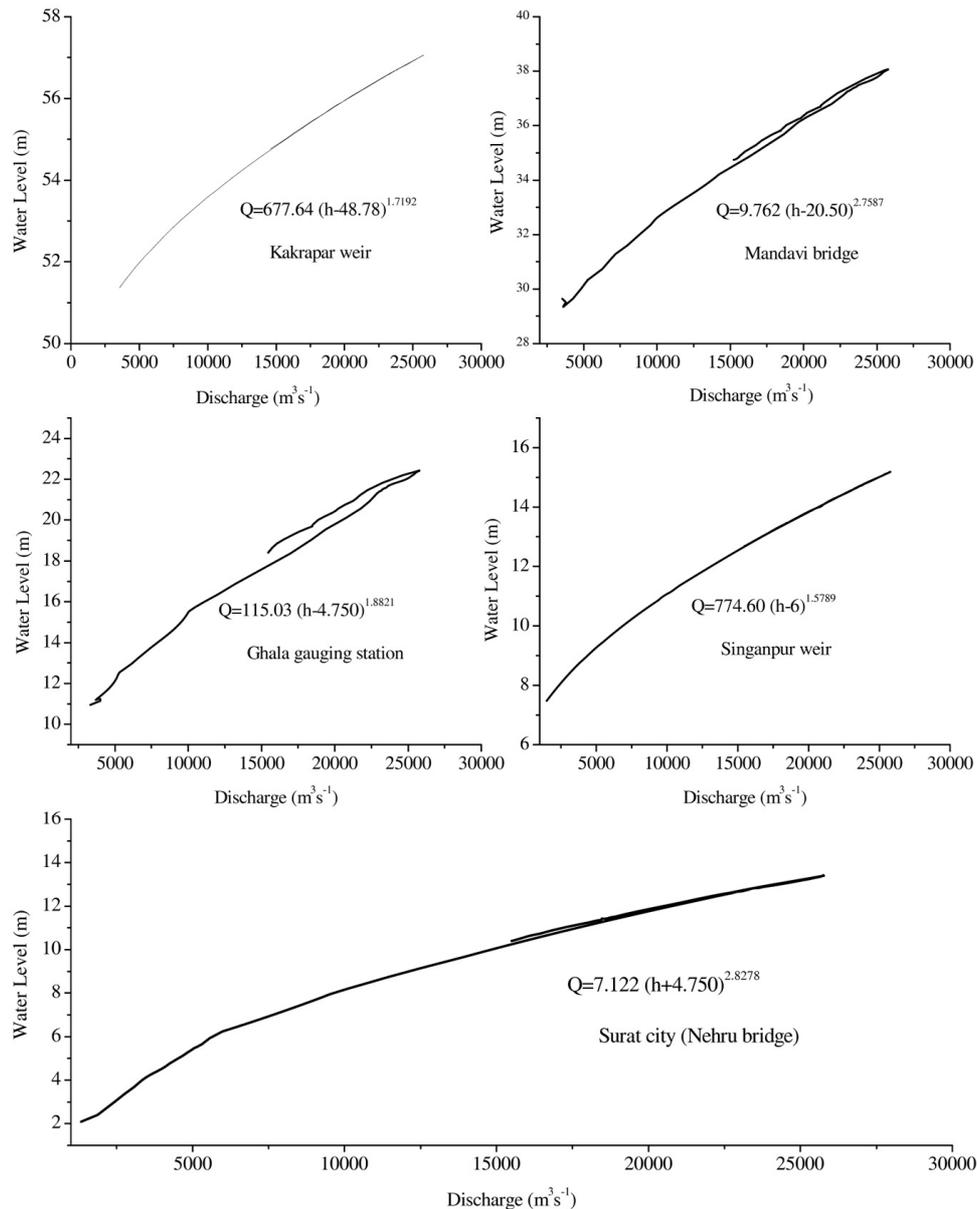
Figure 7. Rating curve (Q–h relationship) along the lower Tapi River.
