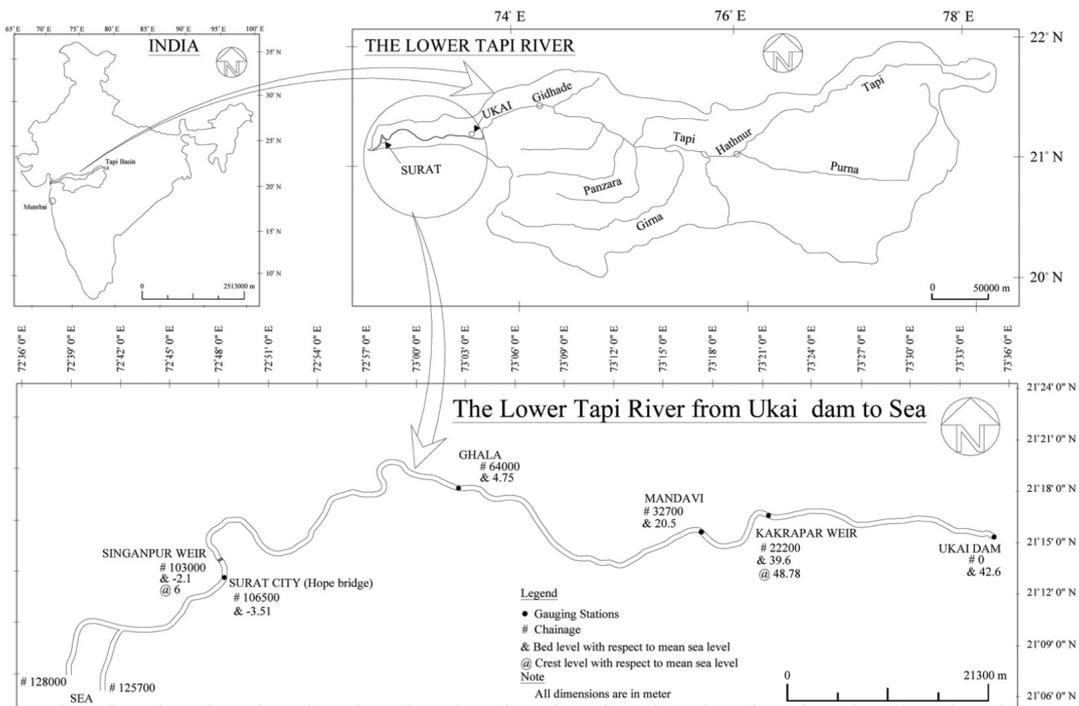
Figure 1. Map of the Tapi Basin, including the study reach in the lower Tapi River<sup>18</sup>.
