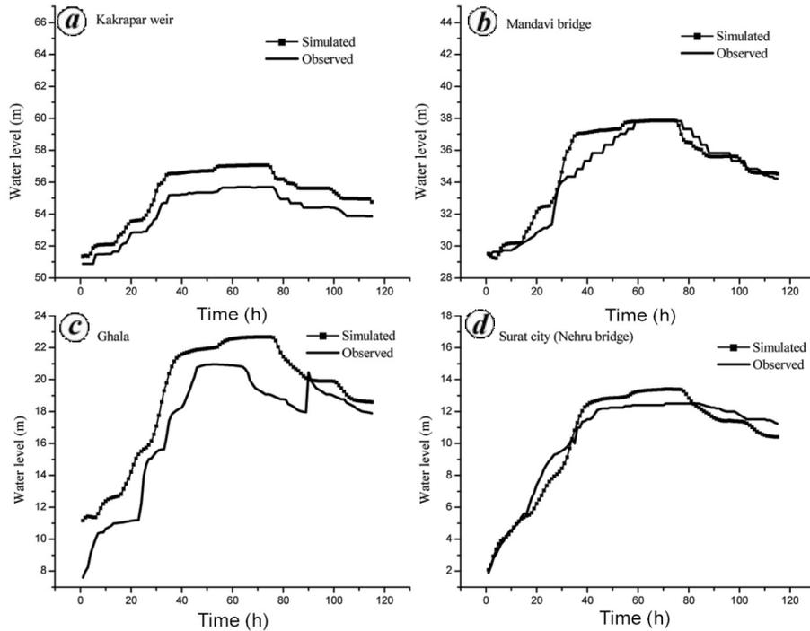
**Figure 4.** Comparison of the observed and simulated stage hydrographs: *a*, Kakrapar Weir; *b*, Mandavi Bridge; *c*, Ghala village; *d*, Surat city (Nehru Bridge).
