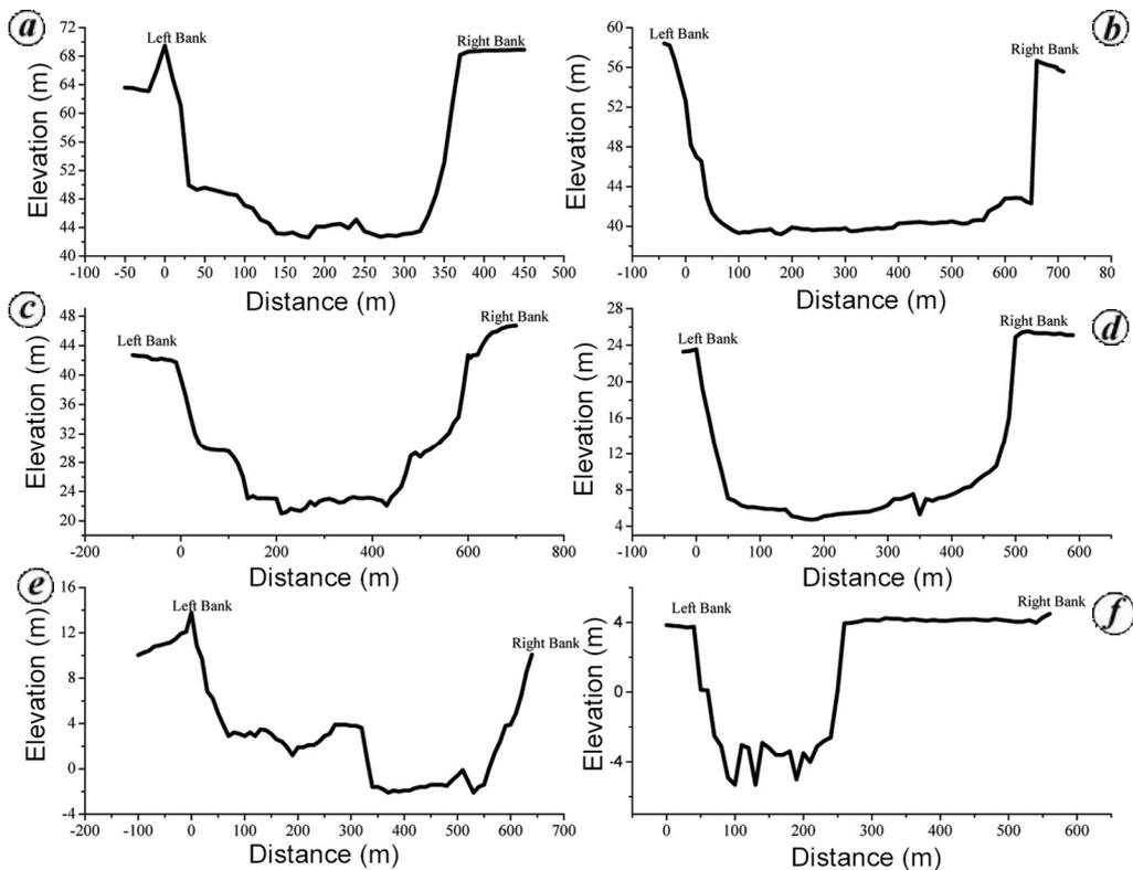
Figure 3. Cross-sections of the lower Tapi River: a, Ukai Dam; b, Kakrapar Weir; c, Mandavi Bridge; d, Ghala village; e, Singanpur Weir; f, Nehru Bridge (Surat city).
