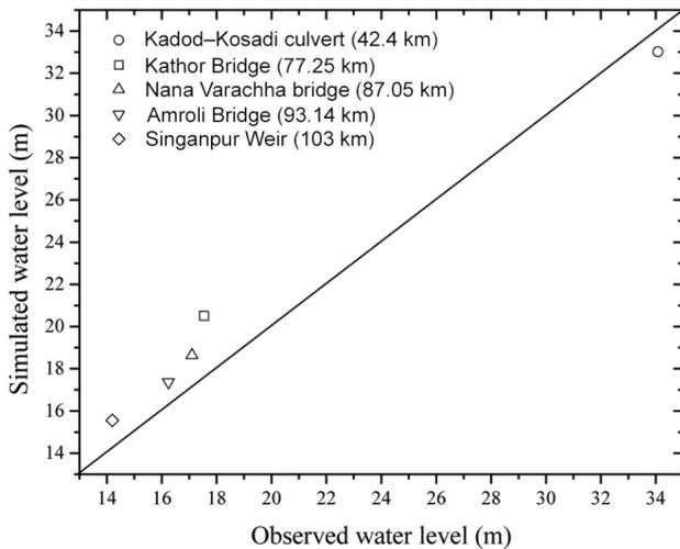
**Figure 5.** Comparison between the observed and simulated highest water levels.
