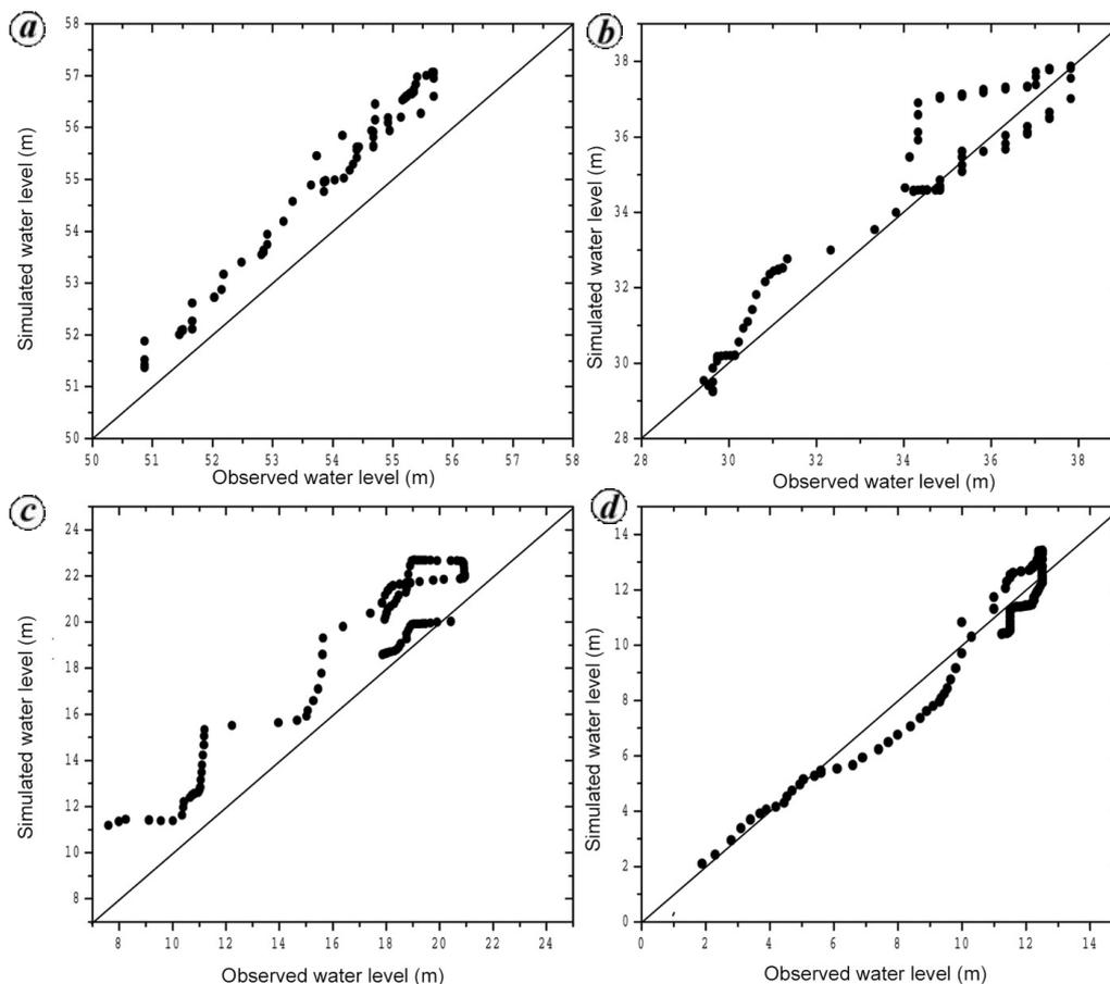
**Figure 6.** Comparison of scatter plots of the observed and simulated hourly water level: *a*, Kakrapar Weir; *b*, Mandavi Bridge; *c*, Ghala village; *d*, Surat city (Nehru Bridge).
