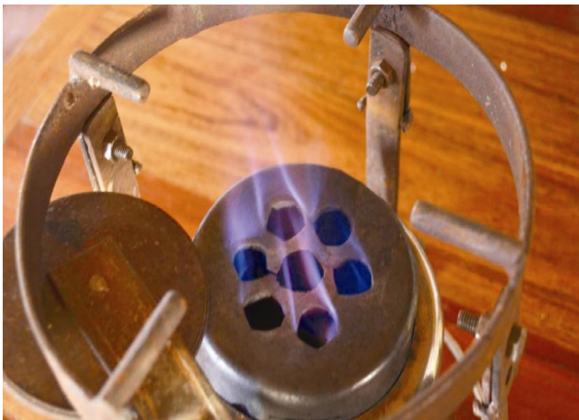
Figure 2. Flame of the VOAHAJA ethanol stove burning 50% ethanol–water mixture without pressure system.
