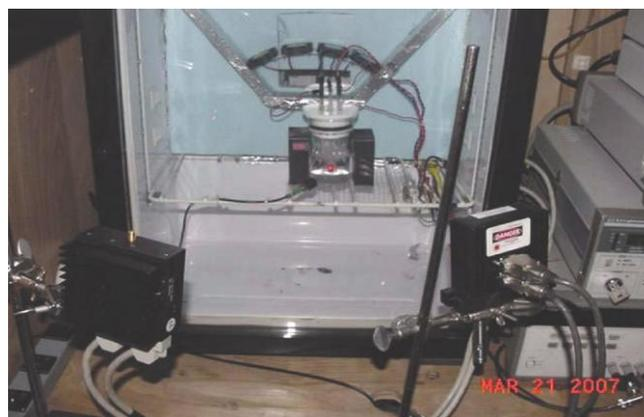
**Figure 2.** Cell inside a temperature enclosure designed to hold ambient temperature at  $25 \pm 0.03^\circ\text{C}$ . A pair of permanent magnets is positioned next to the cell and provides approximately 625 gauss at the cathode. The dual lasers are shown in the foreground.
