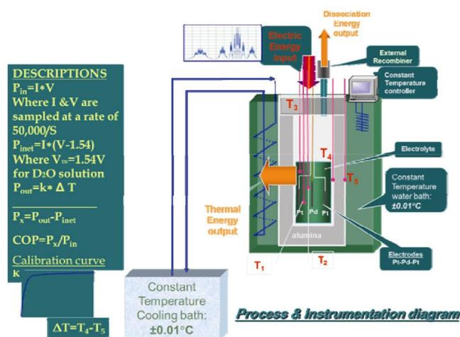
Figure 1. Electrolytic cell with isoperibolic calorimeter.
