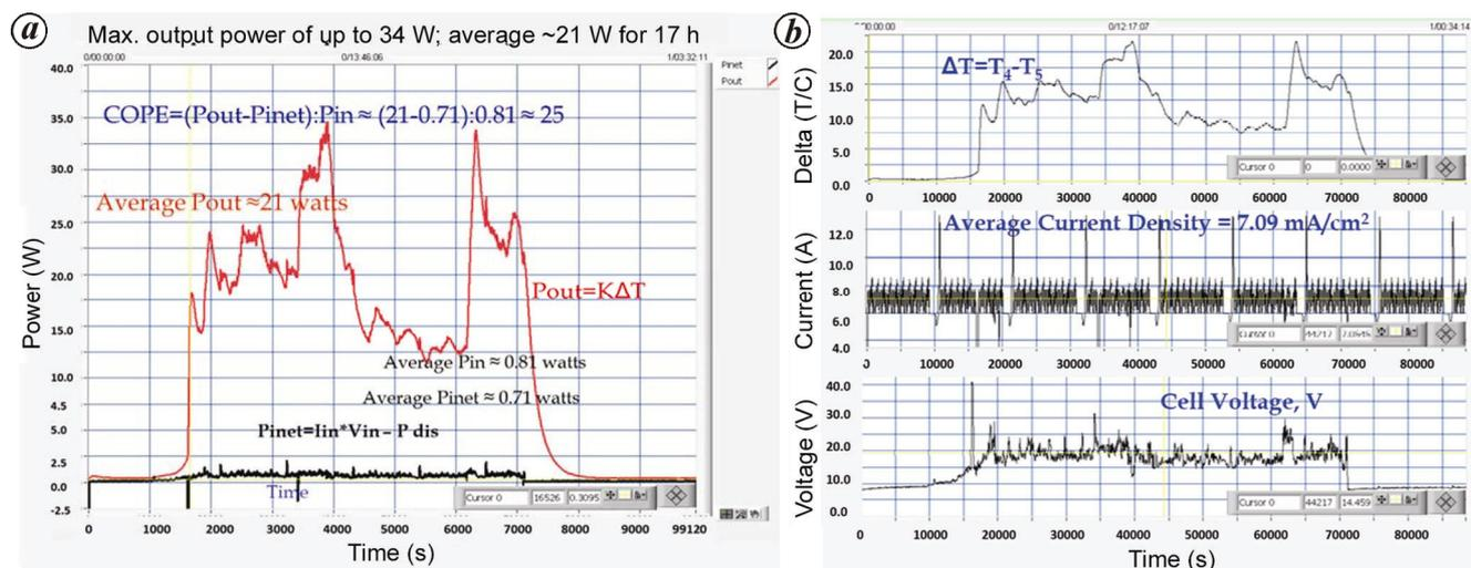
**Figure 3.** Calorimeter results and electrochemical parameters in electrolysis of 0.1 M LiOD/D<sub>2</sub>O. *a*, Excess power (red) versus input power (black). *b*, Currents and voltages of the electrochemical cell.
