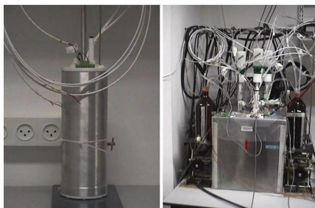
Figure 2. (Left) Electrolytic cell and (right) experimental set-up with three cells in the constant temperature controlled bath.
