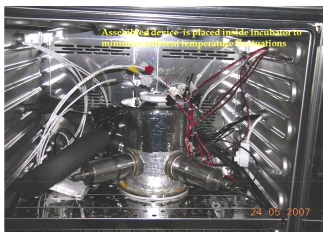
**Figure 8.** Experimental set-up of ultrasound stimulated electrolytic cell (#3) with mass flow calorimetry.
