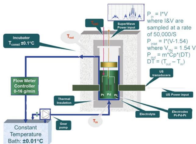
**Figure 7.** Electrolytic cell with ultra sound excitation and mass flow calorimetry.
