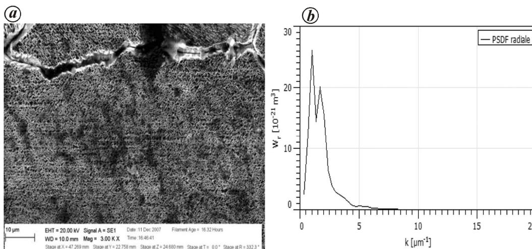
**Figure 6.** Post-electrolysis cathode sample from experiment #64 which had a very large AHE. *a*, SEM image of the cathode. *b*, PSD of the cathode surface structure.
