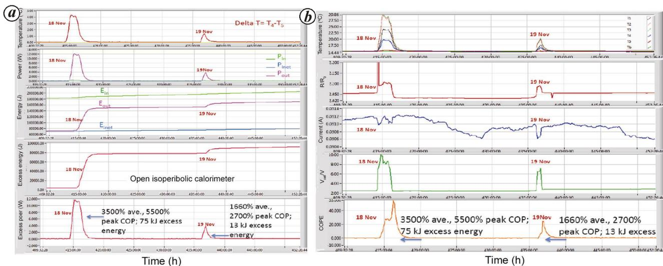
**Figure 11.** Two consecutive excess heat bursts observed during electrolysis of heavy water using a Pd-SWCNT composite cathode. *a*, The measured input and output energies and power, and the calculated excess energy and power. *b*, The electrolytic cell voltages and currents along with various measured temperatures, the resistance ratio of the cathode and COPE.
