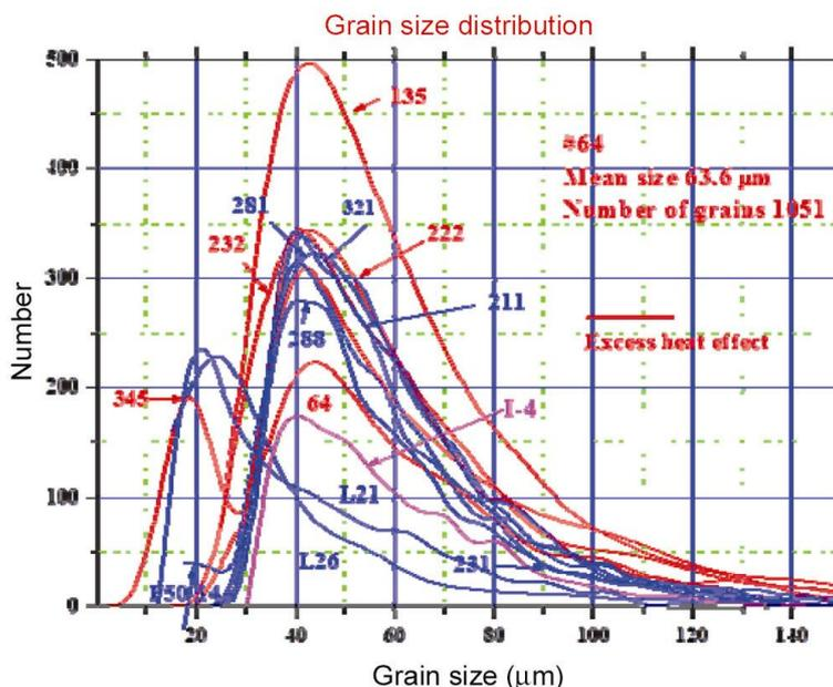
**Figure 5.** Grain size distribution of the cathode from sample #64 compared to other cathodes which either exhibited excess heat (red lines) or did not (blue lines).
