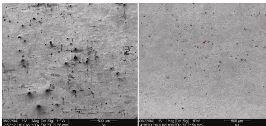
**Figure 4.** Post-electrolysis SEM analysis of foil #63 with no excess heat, and foil #64 (left) with excess heat; both cut from the same rolled strip after rolling and annealing.
