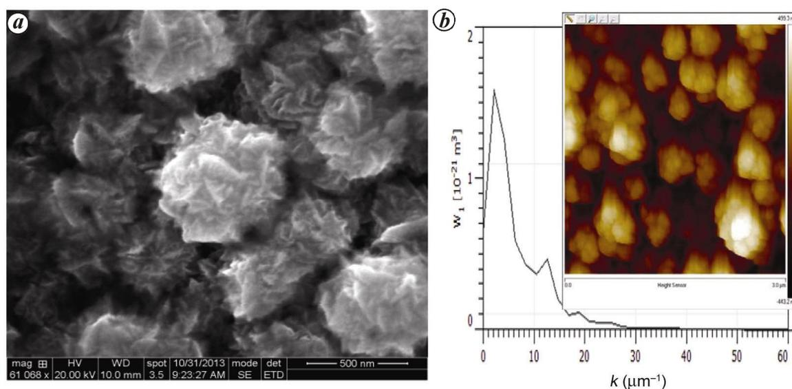
**Figure 12.** Post-electrolysis images of a Pd-SWCNT cathode which yielded excess heat bursts. *a*, SEM image showing the surface morphology. *b*, PSD plot of AFM-measured feature heights across the surface. (inset) Original AFM image.
