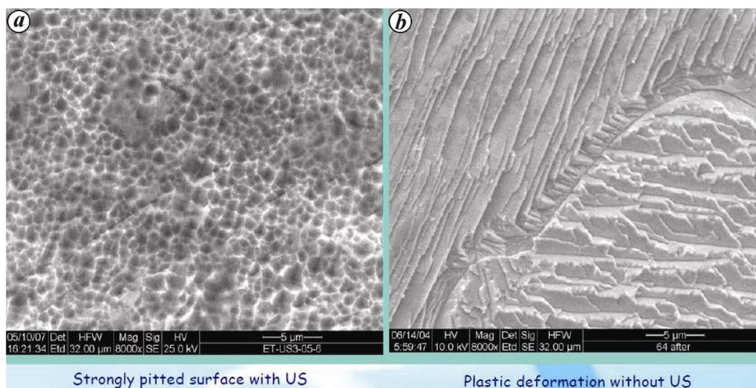
**Figure 10.** SEM images of two palladium cathodes (a) with and (b) without periodic application of ultrasonic waves.
