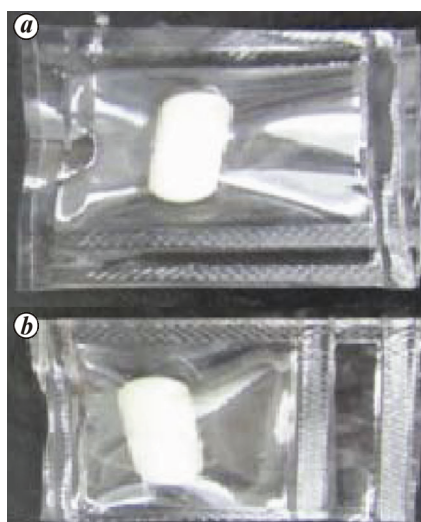
Figure 1. \text{Li}_2\text{CO}_3 powder packed in gelatin capsules and sealed in PVC.
