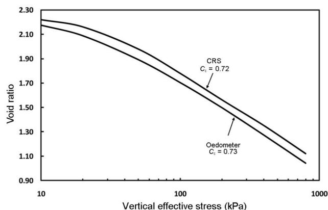
**Figure 2.** Comparison of stress–void ratio relationship of soft soil specimen prepared at 50 kPa slurry consolidation pressure. Specimens collected from Kanjur Marg soil site.
