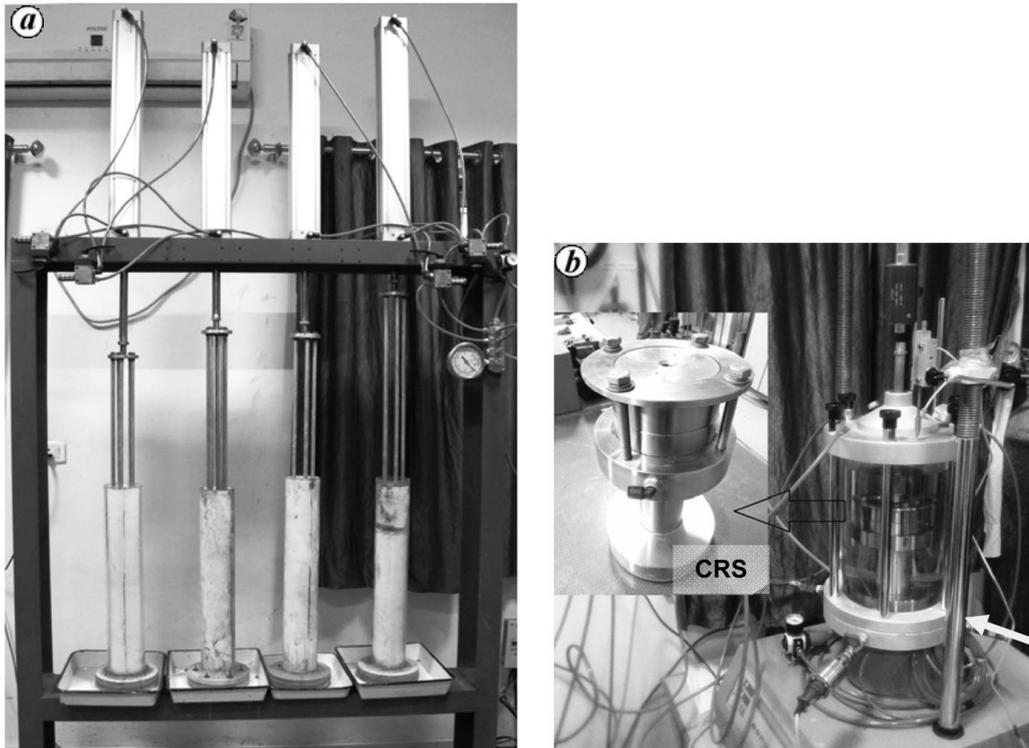
**Figure 1.** Testing set-up. (a) Slurry consolidation set-up (in-house) for preparation of soft soil remoulded specimens. (b) CRS consolidation set-up (in-house) for determination of compressibility parameters of cement-treated soft soil.
