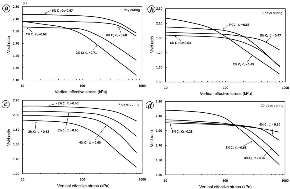
**Figure 6.** Relationship between cement content and compression index of soft soil at different curing periods: (a) 1 day, (b) 3 days, (c) 7 days and (d) 28 days.
