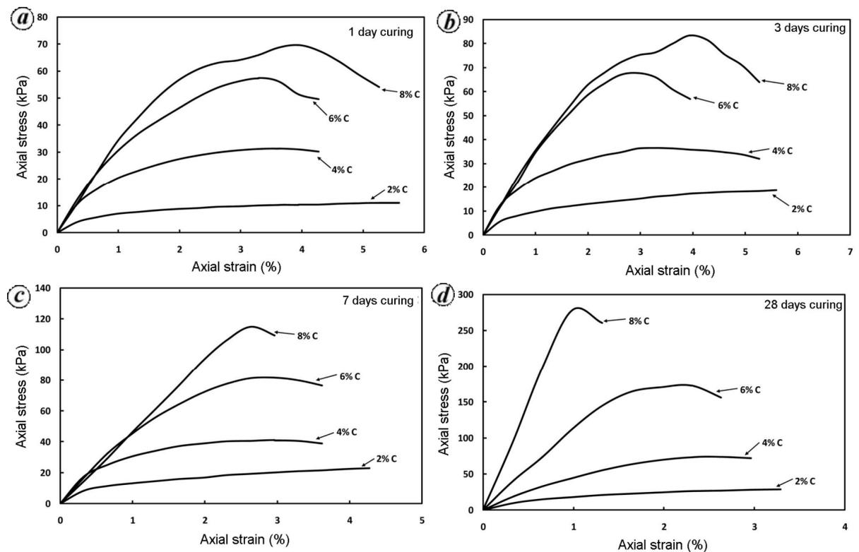
**Figure 4.** Effect of cement content on unconfined compressive strength of soft soil at different curing periods: (a) 1 day, (b) 3 days, (c) 7 days and (d) 28 days.
