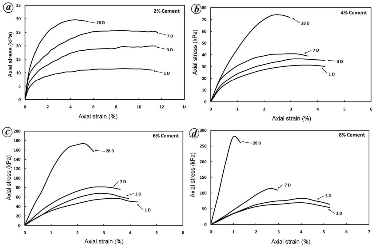
**Figure 3.** Effect of curing time on unconfined compressive strength of soft soil treated at different cement contents: (a) 2%, (b) 4%, (c) 6% and (d) 8%.
