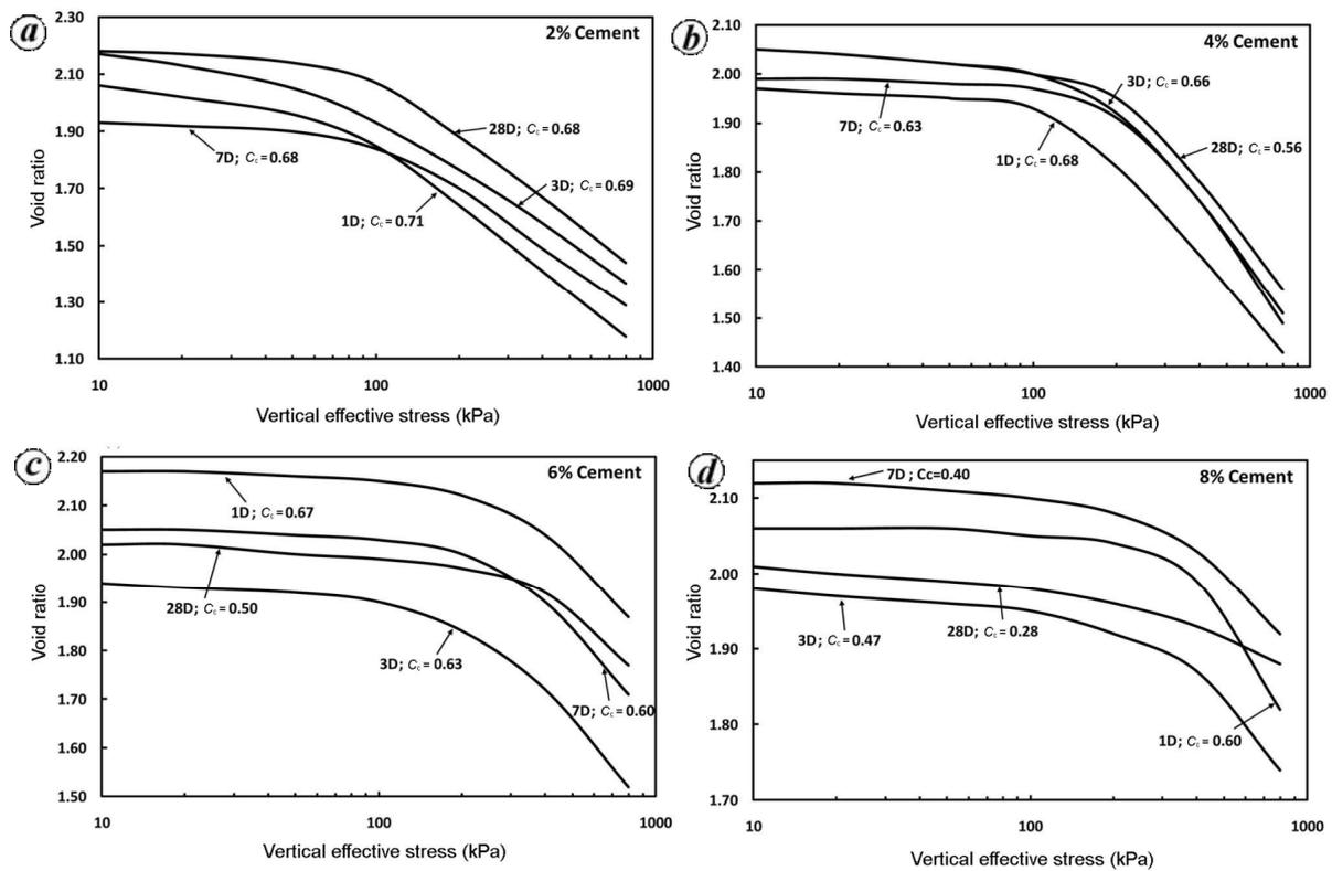
**Figure 5.** Relationship between curing time and compression index of soft soil for different cement contents: (a) 2%, (b) 4%, (c) 6% and (d) 8%.
