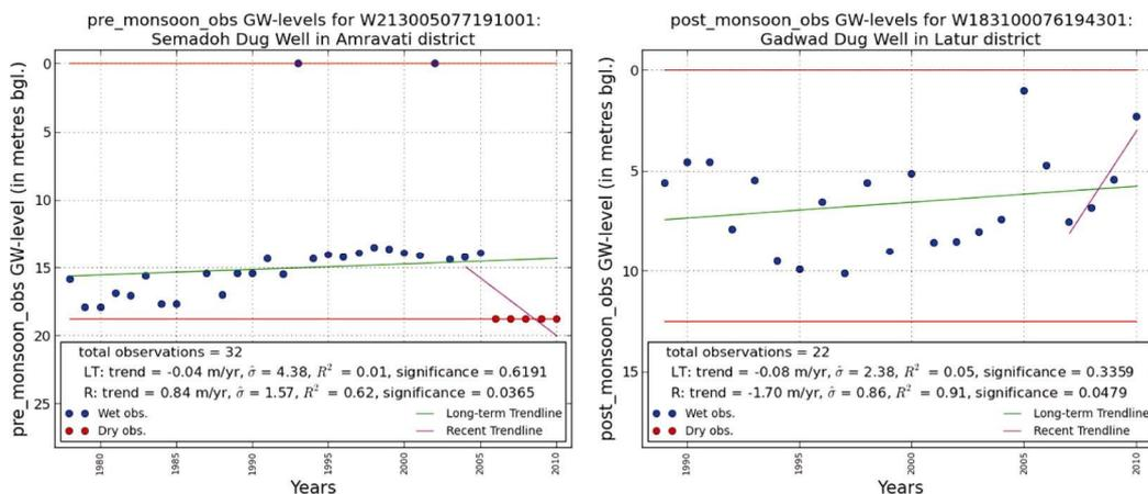
**Figure 5.** Examples of wells with statistically significant trend in recent years, whose long-term trend is GEC-insignificant. Green line is long-term trend (LTT) using GEC'97 and pink line is significant recent trend (RT) using the present algorithm.
