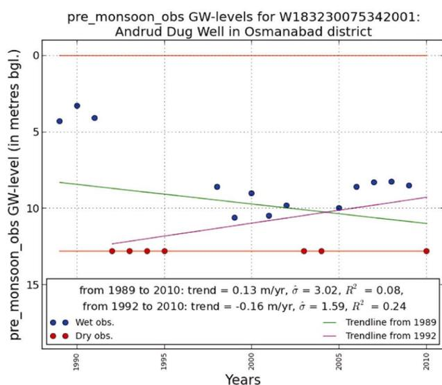
**Figure 2.** Example of dependence of long-term trend on monitoring span.
