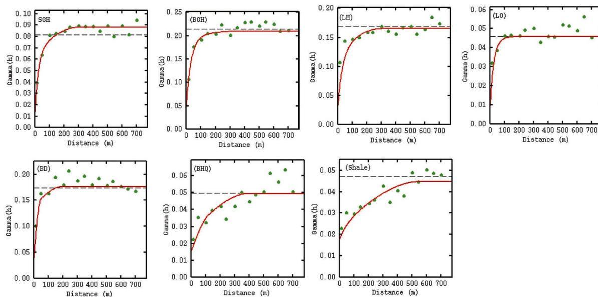
**Figure 4.** Indicator variogram models for each litho type. The variograms of seven litho units show good spatial structure with low nugget values.
