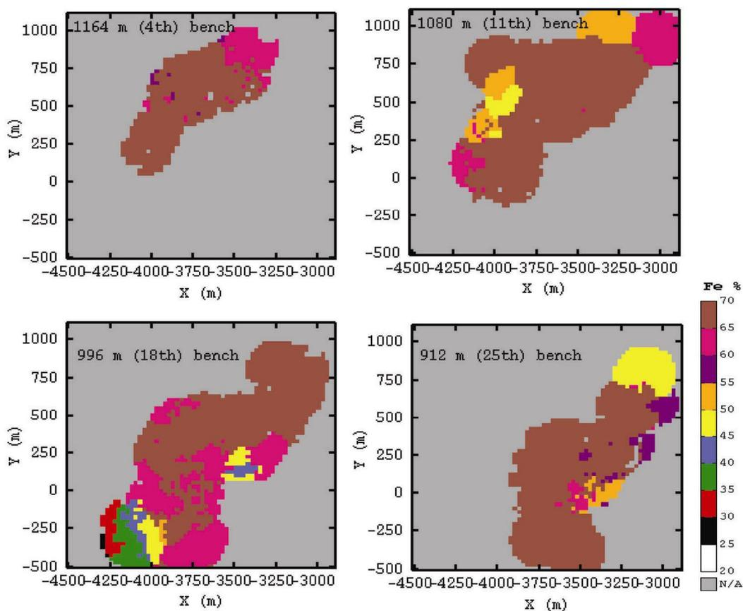
**Figure 8.** Grade maps of four mining benches located at 1164, 1080, 996 and 912 m based on kriged estimates. Majority of the blocks in each bench have estimated Fe >40% and very few peripheral blocks have estimated grade <40%.
