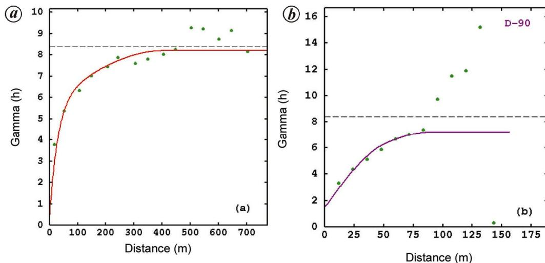
**Figure 6.** Omni-directional semi-variogram models of Fe% for domain A in horizontal direction (a) and vertical direction (b). Both the semi-variograms show good spatial structure with nested models. Small nugget effect is observed in both the models.
