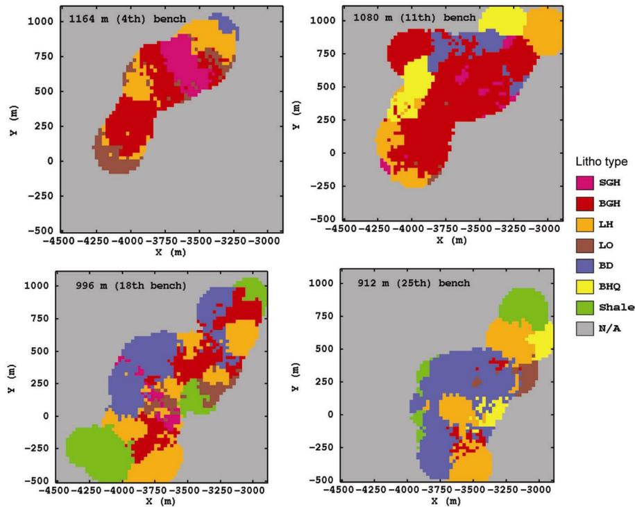
**Figure 5.** Lithological maps of four mining benches located at 1164, 1080, 996 and 912 m. Majority of the blocks in each bench are categorized into high-grade Fe litho units. Banded hematite quartzite and shale containing low Fe grade are observed in peripheral areas.
