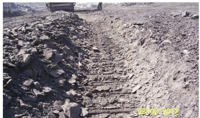
**Figure 2.** Windrowing discharge system of surface miner at SBOC mine, ECL.
