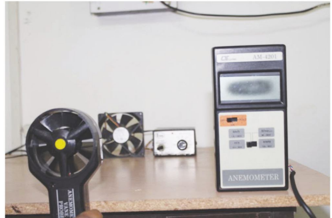
Figure 3. Air speed calibration using anemometer under varying voltages.
