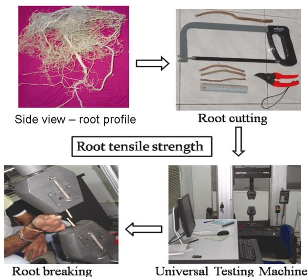
**Figure 2.** Assessment of root tensile strength using Universal Testing Machine.
