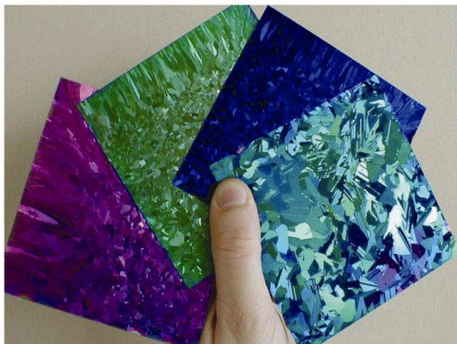
Figure 3. Multi-crystalline silicon solar cells with differently coated (thickness) anti-reflection films on them. Deep blue is the most commonly adopted colour for maximum light absorption. (Source: ref. 1; http://pveducation.org/pvcdrom/design/arc-color ).
