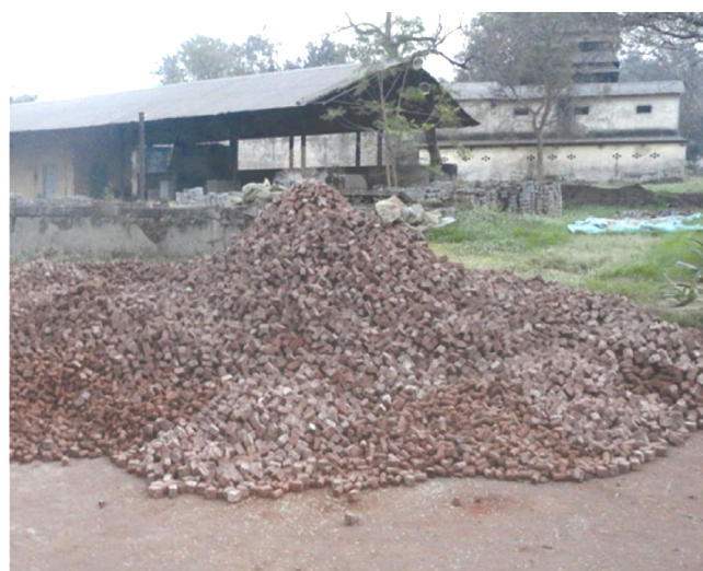
Figure 2. Briquettes produced from slime and used coolant in LD converters.
