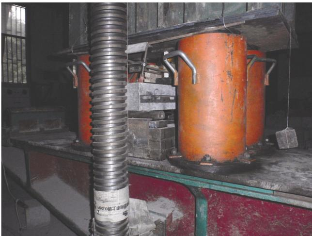
Figure 3. Loading device of three-point bending test.
