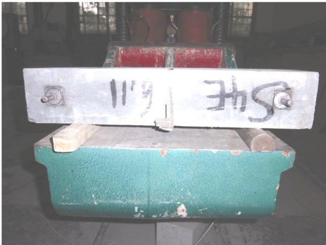
**Figure 2.** Photograph of the beam specimen with pre-cutting crack.
