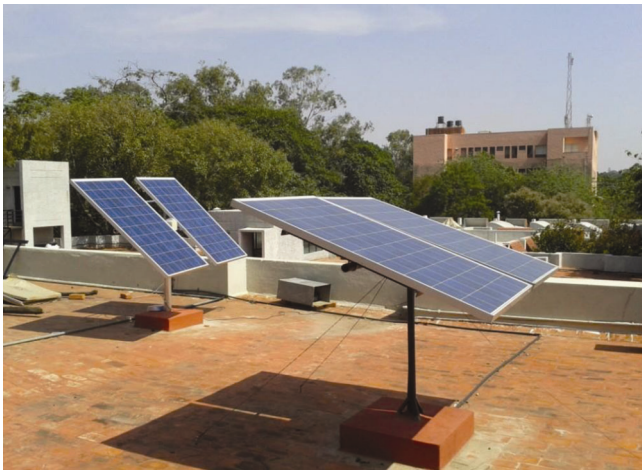
Figure 1. Experimental set-up: (Right) Fixed axis panels and (left) Dual axis panels.
