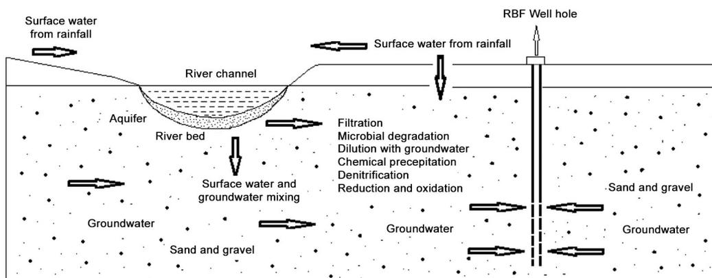
Figure 1. Modified general scheme of RBF<sup>2</sup>.
