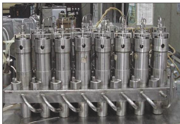
Figure 7. A view of the 16-stage centrifugal extractor bank.
