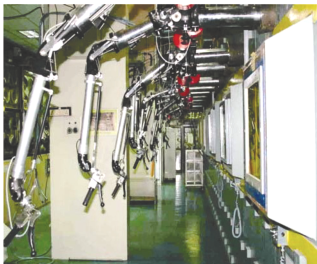
Figure 2. CORAL – hot cell operating area.
