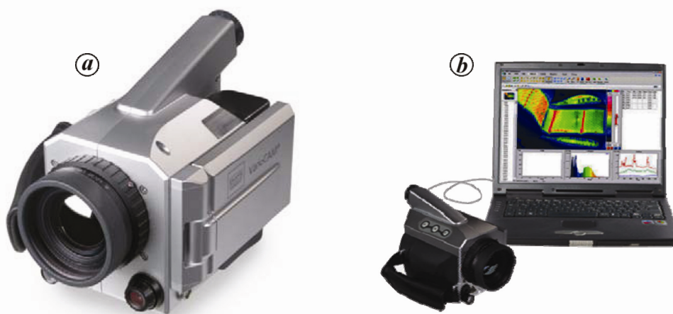
Figure 1. Infrared thermography equipment. a , IR camera; b , Camera and processing laptop.
