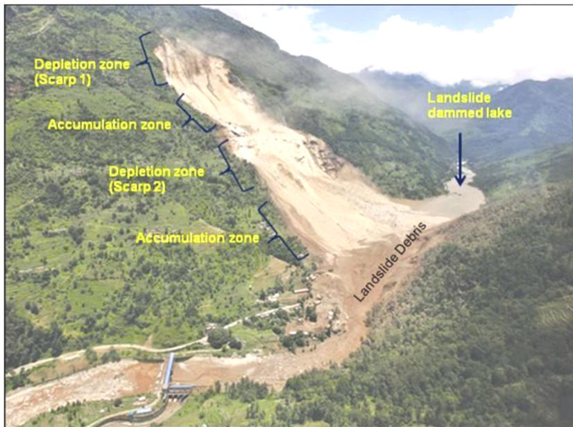
Figure 2. Field photograph of the Sunkoshi landslide (source: [www.ekantipur.com](http://www.ekantipur.com)).
