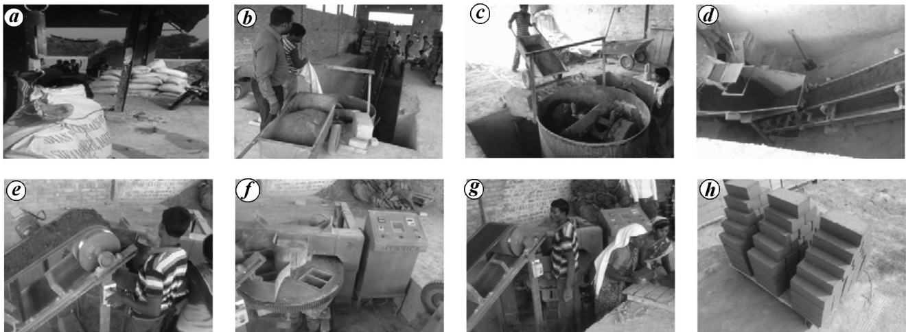
Figure 4. Brick-making process. a , Weighing and batching; b , Feeding of raw material; c , Mixing of material; d , Mixing unit to hopper; e , Hopper to conveyor; f , Conveyor to brick mould; g , Stacking of wet brick; h , Final brick after curing.
