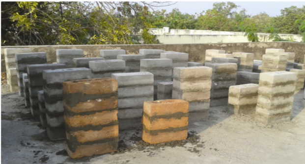
Figure 5. Photograph showing three-brick and five-brick prism for compressive strength, shear bond and flexural bond test.
