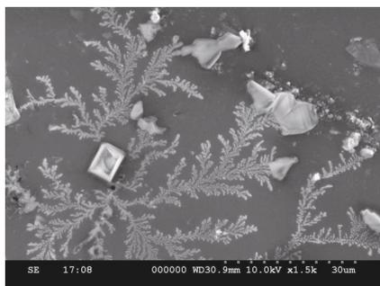
**Figure 4.** Fractal formation of silicic acid in aqueous tetrahydrofuran medium: an SEM image of the imidazole initiated fractal structure of silica.
