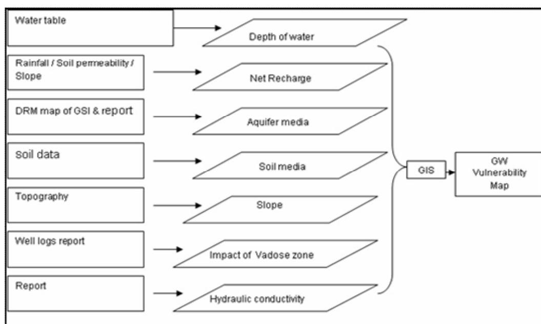
**Figure 3.** Methodology for groundwater vulnerability analysis.
