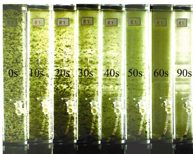
Figure 3. Composite images of reactor showing separation of granular biomass from bulk. Number in each column shows the time (sec) after the stopping of aeration.
