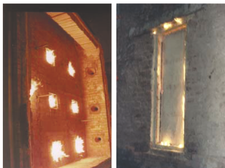
Figure 6. Testing of fire door in the furnace.
