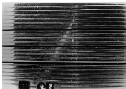
Image of a shower due to interaction of hadron in the Big Multi-plate Cloud Chamber in the experiment at Ooty (Courtesy: J. Acharya, Photography Section, TIFR).
