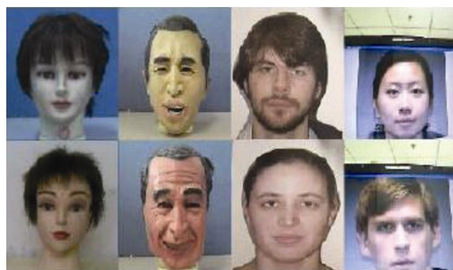
Figure 1. Examples of fake facial specimens. From left to right columns are silica gel, rubber, photos and video replay 2,3 .
