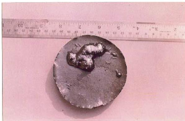
Figure 4. Four inch diameter multi-crystalline Si ingot from rice-husk (adapted from ref. 10).
