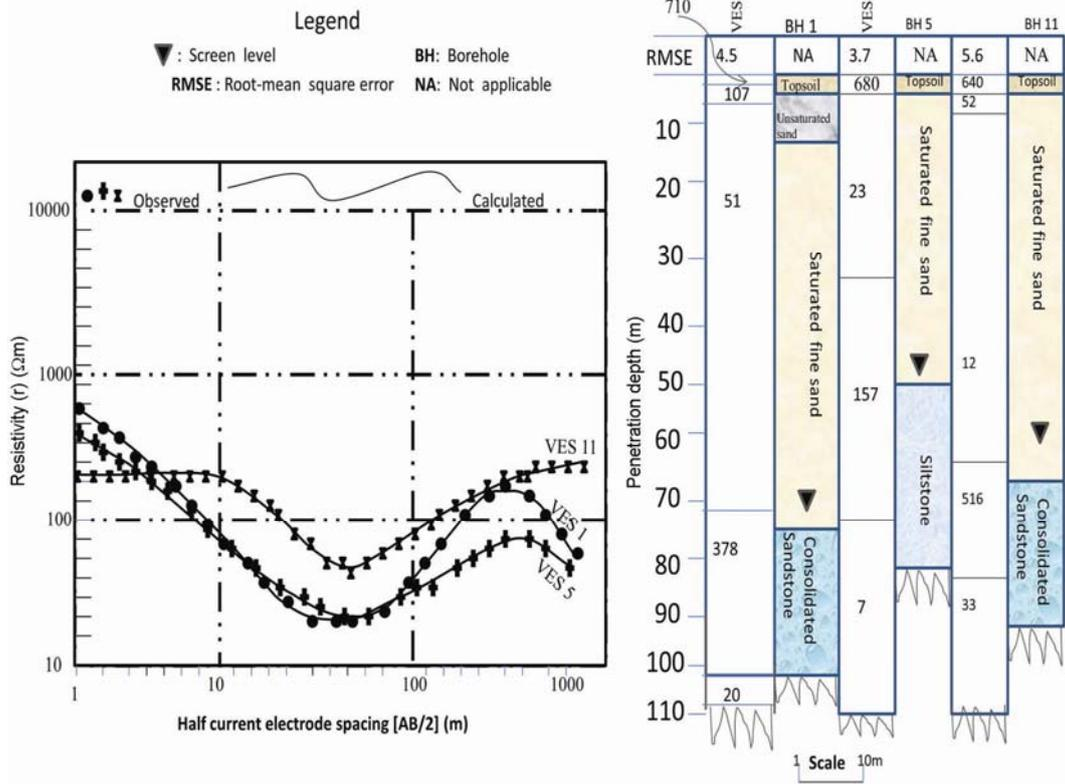
Figure 2. Samples of 1D-derived modelled VES curves correlating with nearby borehole lithologies in the study area.
