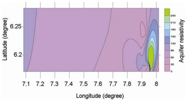
Figure 3. Contour map showing distribution of aquifer bulk resistivity in the study area.
