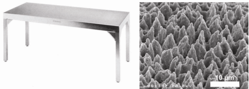
Figure 1. A steel table looks smooth. However, an electroscopic image of steel (10 μm) is not smooth.
