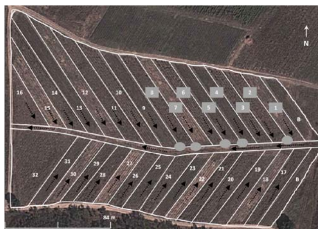
Figure 1. Layout of the experiment. Numbers represent plots. Filled rectangular boxes represent plots with soil water monitoring setups, filled circles represent plots with runoff recorders and black dotted arrows represent direction of runoff flow.
