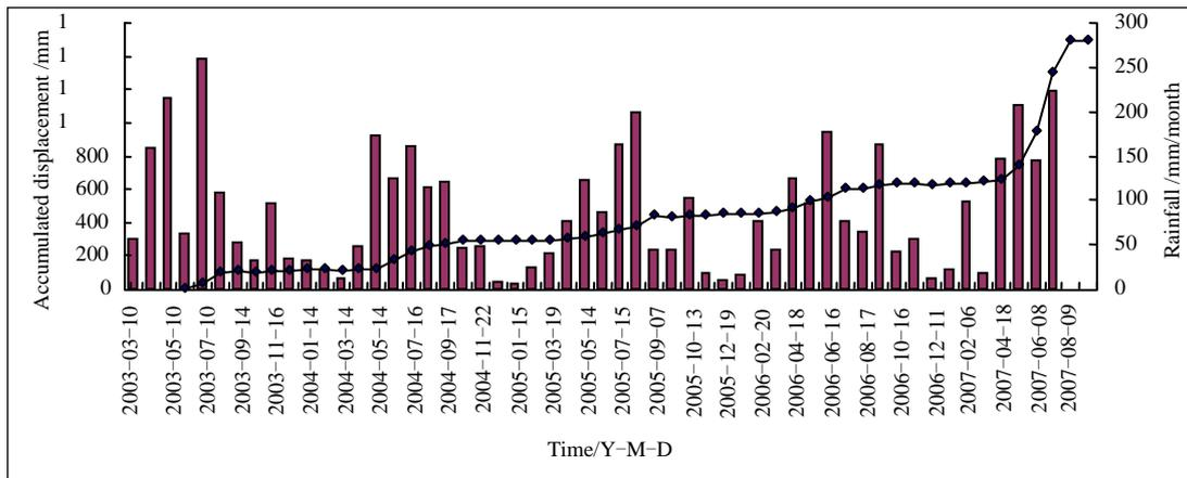
**Fig.1** Stepped deformation curve of Baishuihe landslide in Three Gorges reservoir
