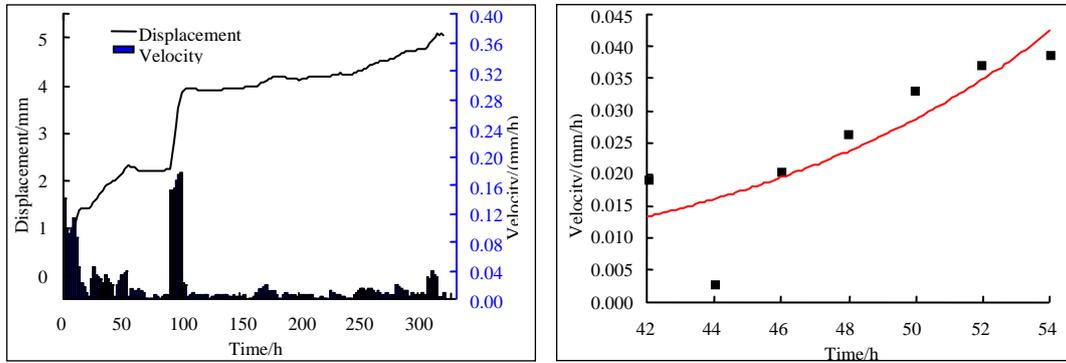
Fig.6 Sample TR-3 rheological experimental curve
