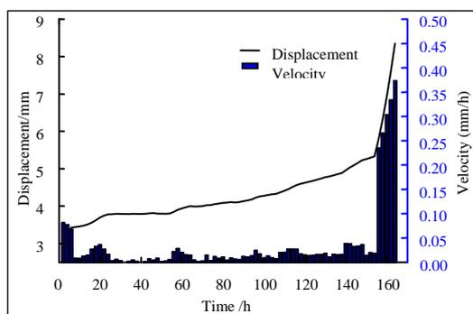
(a) Cumulative displacement and deformation velocity
