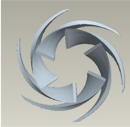
*Fig.3 Blade model of the runner*
