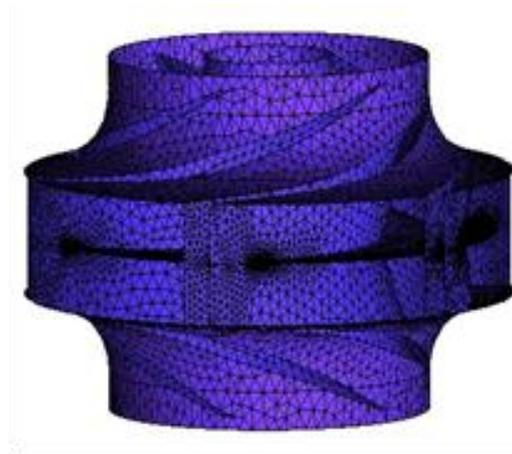
*Fig.5 Mesh dividing of integral impeller*
