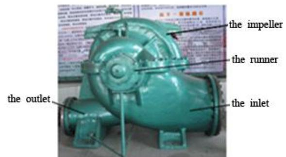
Fig.1 Double-suction centrifugal pump for 1200s-56
