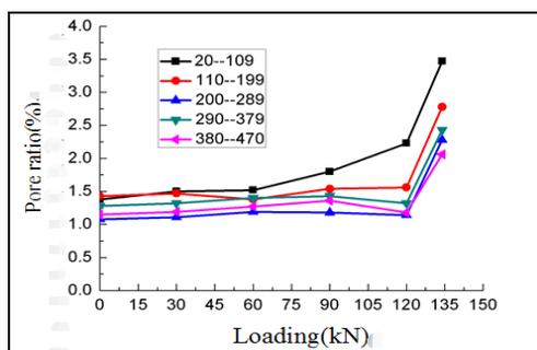
**Figure 8:** Pore ratio change with loading
