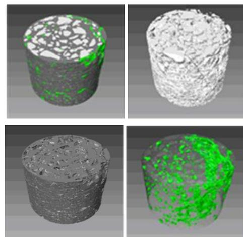
Figure 5: From left to right: test specimens, aggregate, mortar, spatial distribution of cracks
