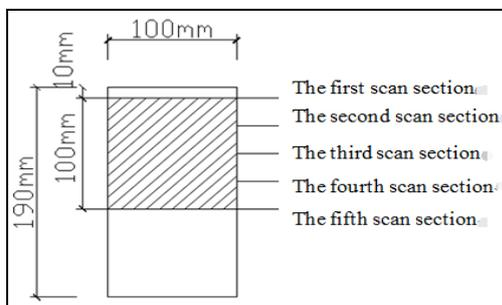
Figure 3: Concrete sections map of CT scan
