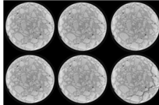
Figure 4: CT scanning images of concrete in different loading
