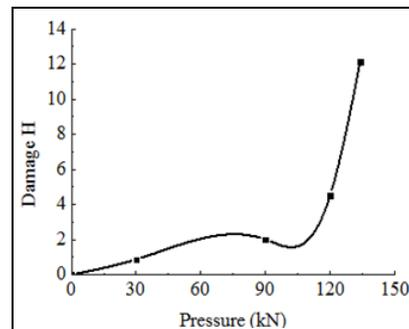
**Figure 10:** Pressure-damage curve of concrete test specimen
