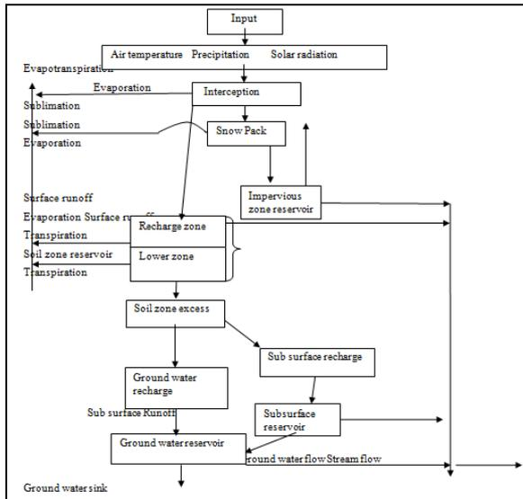
**Fig.2.2.** Schematic presentations for different components of PRMS model (Source: Leavesley et al., 1983) [6].
