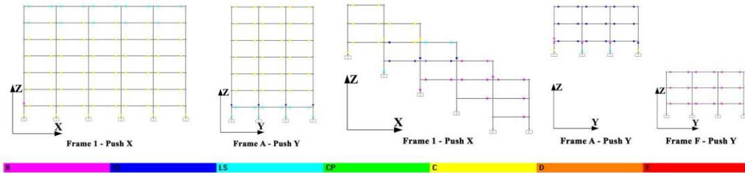
Figure 25: Hinge states in the Type B and Type B1 configuration
