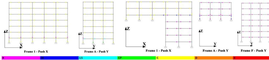
Figure 26: Hinge states in the Type C and Type C1 configuration
