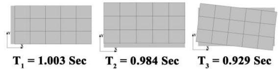
Figure 10: Mode shape of Type C1 configuration
