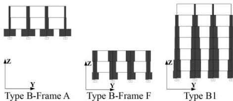
Figure 15: Variation of column force along the height for earthquake force along Y-direction
