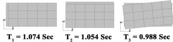
Figure 6: Mode shape of Type A1 configuration
