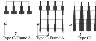
Figure 16: Variation of column force along the height for earthquake force along Y-direction
