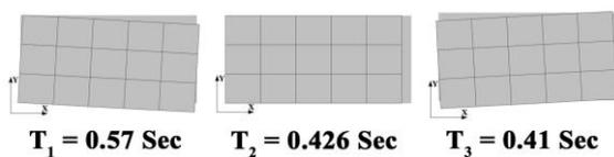
Figure 9: Mode shape of Type C configuration
