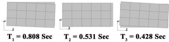
Figure 5: Mode shape of Type A configuration
