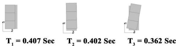
Figure 7: Mode shape of Type B configuration
