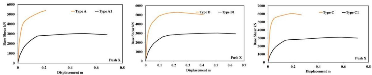
Figure 27: Comparison of capacity curve for push along X direction
