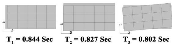
Figure 8: Mode shape of Type B1 configuration
