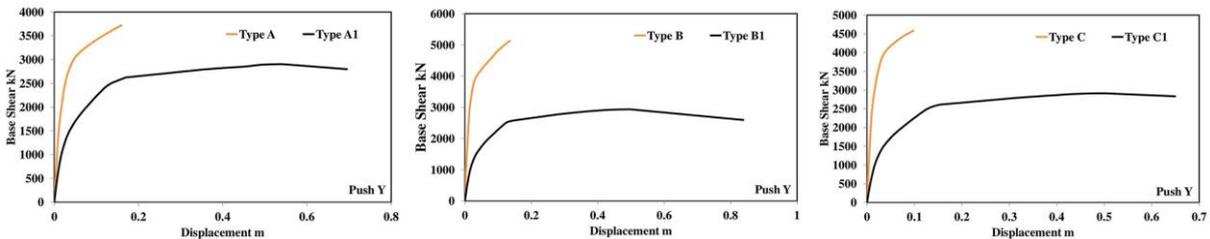
Figure 28: Comparison of capacity curve for push along Y direction
