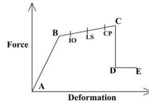
Figure 23: Force Deformation Plastic Hinge
