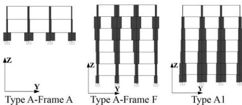
Figure 14: Variation of column force along the height for earthquake force along Y-direction
