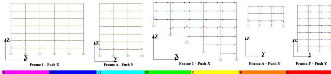
Figure 24: Hinge states in the Type A and Type A1 configuration
