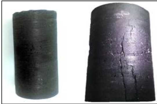
Fig. 2 (a) Sample 1 (Intact) Fig. 2(b) Sample 2 (Visible Crack)
